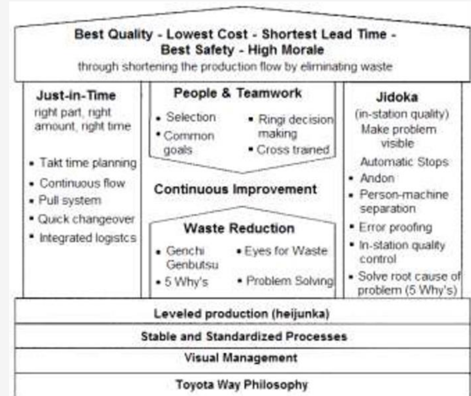
The "TPS House" Diagram : A system based on a Structure , Not just a set of techniques
